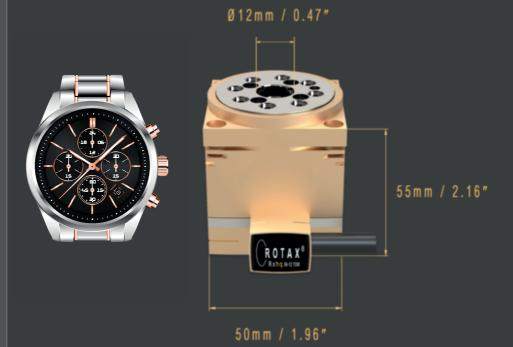
The new miniature hollow shaft servo motor ROTAX® Rxhq (High Torque) impresses with its extremely compact design, extra large hollow shaft and enormous torque. Direct drive motor, precise bearings and the single turn absolute encoder are completely integrated.
